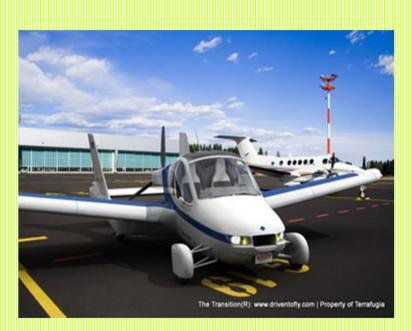
The world's first light roadable aircraft has been officially approved, and the in-line production will begin in the near future. It takes Terrafugia's *Transition*30 seconds to convert from a normal car into a two-seat light aircraft. Taking off with a full tank, the vehicle has a flight range of 644km and a cruising flight speed of 185km/h. To take off, the aircraft needs a 500m long runway, and it has a load capacity of approx. 200kg.
