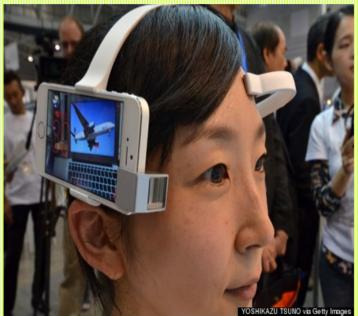
wish you'd been holding a video camera? Japanese tech company Neurowear's high -tech headgear, Neurocam, aims to solve that problem for you. The device straps a camera and an electroencephalogramreader to the wearer's cranium. During moments of high-frequency electronic signals detected through the skull - a general indication of excitement the camera switches on to record short fivesecond GIFs onto an iPhone that is somewhat awkwardly attached to the device.
